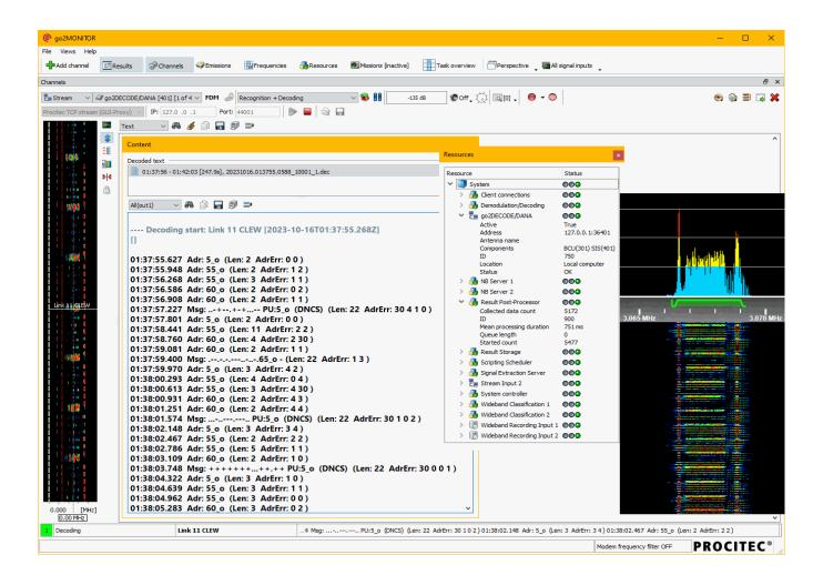
3067.8 kHz Digital data station using the NATO Standard Link-11 (CLEW) system
